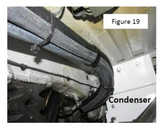
12. The heater hose marked with red tape is cut, attached and clamped to the output of the Water Valve. The other end is attached to the input of the Booster Pump and routed to the engine compartment (Figure 20). The second heater hose runs from the Evaporator Out to the engine compartment. A third heater hose (62 000 274) should be marked with orange tape (or in some other way) and is clamped to the Wye between the Booster Pump and the Water Valve and runs to the engine compartment (Figure 21).
