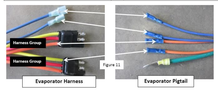
Cut off the connectors on the harness and strip to bare wire. Blue goes to Blue (doesn't matter which one to which one). The orange of one harness group and the yellow of the other group go to the orange pair on the pigtail in either order (Don't use the yellow and orange from the same harness group)(Figure 11). The Evaporator Pigtail has butt connectors already attached. Crimp connections and wrap the bundle with electrical tape.
